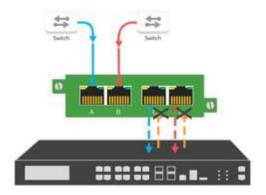
Data Diode SPAN TAP
